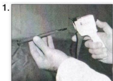
Raise slide release lever on dispenser body and insert piston slide.
