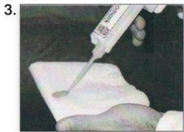
For new cartridges only, dispense a small amount of compound on to waste paper.
