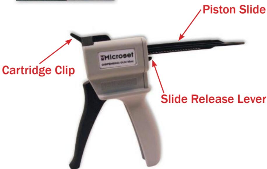
MICROSET is supplied in a two part cartridge which is dispensed through a static mixing nozzle using a hand held dispenser. The two components of the cartridge are mixed together as they pass through the static mixing nozzle during the dispensing procedure. This ensures air-free mixing and minimum wastage of material during application.
