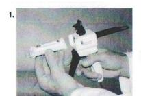
Lift cartridge retaining clip on dispenser body and position cartridge.
