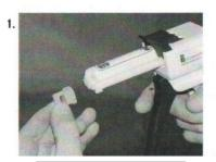
Rotate cartridge cap counter-clockwise ¼ turn and pull to remove.
